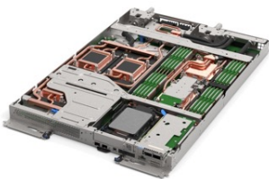
Figure 2 | Lenovo® ThinkSystem™ SD650 V3 server tray showing the direct-water cooling (DWC) module
